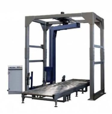
Sensor test pallet height, can design different wrapping modes Soft start/stop, home position,
