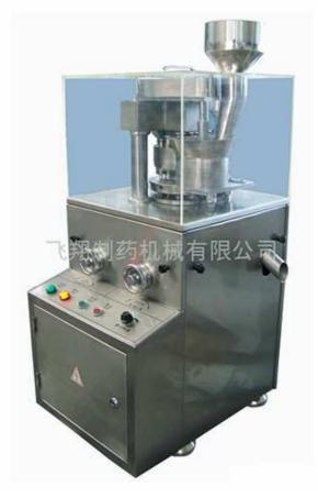
ZP9D Rotary tablet press is a new generation product by our factory, and this machine is a single roller continuous automatic tablet press for pressing various kinds of different shape tablets and plain tablets, such as round tablet, irregular tablet and carved tablet etc.
