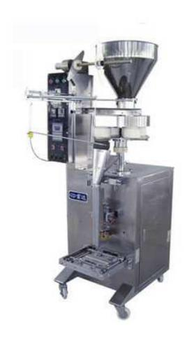
This granular packing machine can automatically finish the processes of bag making, metering, filling, cutting, counting and batch number printing. The machine is equipped with high-speed printer to automatically print the batch number, storage life, etc.
