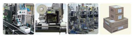
PA6000 enables real time printing and application of labels on to product packages. Information such as production data, serial & batch numbers, anti-counterfeit numbers, unique product ID, packaging data, and distribution channel data etc. can be printed to the label in characters, barcodes, or 2D codes, or even in the form of RFID. Automatic application of these information online enables effective track and trace of the products in the subsequent distribution channels.
