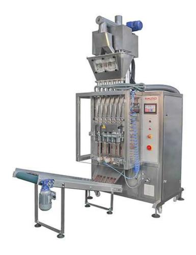
This fully automatic filling machine is designed to pack untouched, affixed-on-three-sides packets like coffee, coffee cream, energy drinks, medical powder that has no spontaneous fluency through screws by disposable products. Non free flowing powder products can be packaged with this machine using screws synchronized with PLC in a high level of sensitivity. The machine can produce 90 pcs/min using 3 channels and 180 pcs/min using 6 channels.
