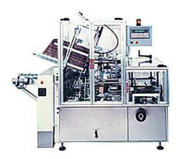
It is a kind side load case packing machine. The machine is designed for arrange number of product into corrugated paper case, product like, medical box, syrup box, CD box... detail as showing.
