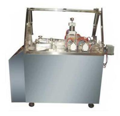
Description: ZD-I model fully automatic suppository belt making machine is the forming equipment that make piece material into bullet head (torpeto), duck mouth type suppository packing belt by feeding, pre-heated, welding, heating froth forming, making split line, cutting bottom side of triangle. It is the first select equipment of product line.
