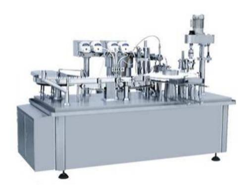
Eyedrops liquid filling and rotating cap machine is a new product that our company developed and researched in recent years. Computer control wriggle pump to measure filling. It has many functions of auto adding inside, capping, rotating-cap, It is the new generation equipment of eye drop production of pharmaceutical industry. The machine can also be used to the production of filling, adding stopper, rotating cap and labeling small dosage liquid in other industry.
