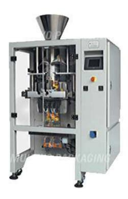
The MK-505 is a High speed servo driven vertical form, fill and seal packaging machine designed to package various whole foods, grains and snack products. This servo driven VFFS packaging machine is equipped with servo drive and it uses 2 to 5 linear weigh scale to produce center sealed pouches also commonly known as pillow pack or fin seal type pouches / bags.
