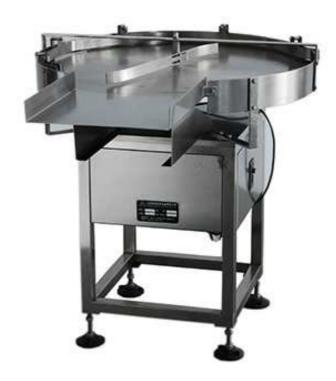
The Unscrambler manually bottle into the round on the turntable, the turntable rotating the bottle continued dial-in conveyor belt, into the filling machine for filling. Easy to use, simple operation, is an indispensable link.
