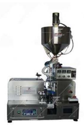
Semi automatic toothpaste tube filling machine cosmetic with mixing and heating system is suitable for package the material which need heating and mixing.
