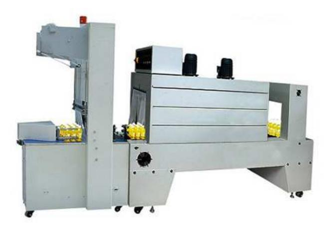
ZJ5038 series sleeve wrapper is suitable for wrapping pop-cans, bottles etc. It works with PE shrink tunnels.
