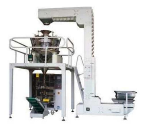
Granule Packing Machine is suitable for pharmacy, food, household chemicals, plastic products and other special industry and other loose type and in viscid granule material. Such as seeds, Chinese Drugs, feeding stuff, medicinal granules, pillar, monosodium glutamate, salt, sugar, soup blend, oat, tea, active carbon, washing powder, dryer, etc.
