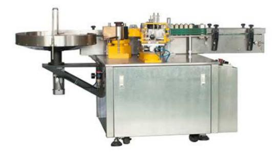
JHL-10 is suitable for small cylindrical container such as glass, plastic, PET bottle with precut paper label. The machine is economical and easy to operate. The performance is stable with a level off and good looking labeling result. The control system adopts convert motor system, the in line conveying bottle, supplying glue and label automatically. This automatic labeling system is ideal for food&beverage, medical industry, etc.
