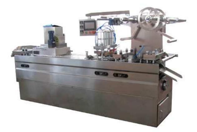
It is the newest high precision capsules and pills/tablets packing machine in current pharmacy industry. It is widely used for capsule, tablet, honey pills in pharmaceutical industry, for milk tablet, candy, chocolate in food industry, for injector, syringes, pins, small component ect. In electron or hardware industry as all kind of shapes of ALU-ALU, ALU-plastic, paper-plastic combined packing.
