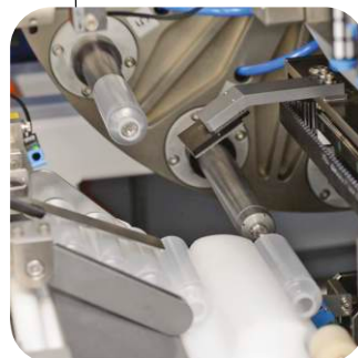
TUBE LOADING STATION
