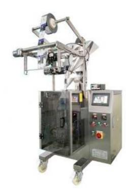
This machine adopts correcting system controlled by microcomputer; owing to a response signal is handling and pass through microcomputer. It can accomplish whole set to synchronization, sack length, position fixing, voluntarily follow the tracks of light-mark and voluntarily diagnose trouble and show to screen.
