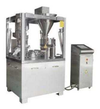
NJP-2000C automatic capsule filler processes the products for optimal productivity up to 2000 capsules per minutes, featuring low-maintenance operation, minimal downtime, and overall dependable production.
