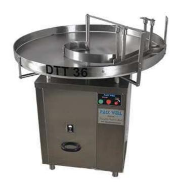
Stainless steel scrambler & un scrambler, which is familiar as turn table. This is built on SS square frame, solid guide rail & reduction gear box for jerk less & noiseless performance. Turntable is useful to ensure total synchronization, uniform flow of container and to take a turn at 90 degree to suit different machine and purpose in automatic liquid line.
