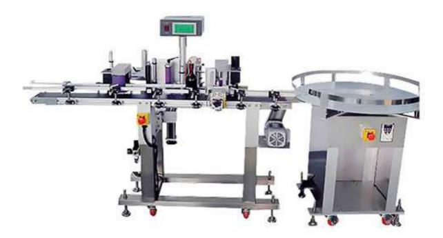
Automatic Labeler, ALR-130 is easy to install & fit label roll. ALR-130 can connect with production line. It is installed touching scree. The Thermos Transferring Print Coder is one of its options.
