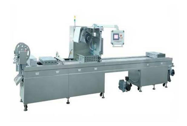
It is called double aluminum film vacuum packaging machine. Double stretch wrapping machine fill the blank of only one side stretch wrapping machine to satisfy the need of aluminum foil packaging products demand.
