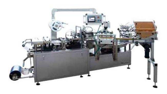
This blister packing machine which is suitable for "PVC/PET blister + Card" packaging for such as battery, glue, lipstick, pen, injection, toy gun, buring torch, toy car, scissor, alarm, toothbrush, coat & hat hooks, chopsticks, cleaning balls, bottle openers and so on.
