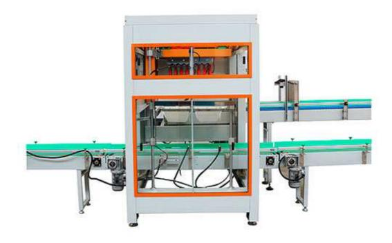
$\star$  The machine grabs the product through the grabber and puts it into the carton to complete the required packing action
