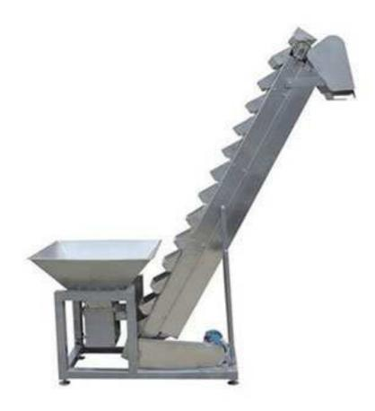
A tilted type bucket elevator is an inclined mechanism for hauling flowable granular bulk materials (most often grain or fertilizer). Usually used as auxiliary equipment for granule filler machine.
