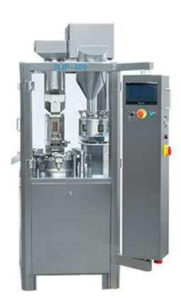
NJP-200 Full automatic capsule filling machine is a full automatic hard capsule filling equipment with intermittent operation and hole plate filling.
