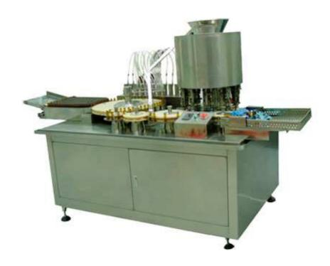
This high speed filling and sealing machine is specially designed for filling, capping and sealing 10ml and 20ml linear bottles with easy open lids or aluminum-plastic lids. Meanwhile, it is the main equipment of the oral liquid production line.
