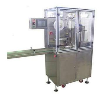
Suitable to piling up thin medicine box with many layers and rows with little kinds boxes, advanced technology, non-shrinking, save 9000W/hour, this machine is the choice instead of middle box in the field of medicines
