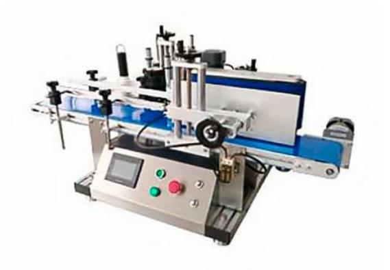
FF-F130 automatic round bottle labeling machine is applicable for labeling various round surfaces made of glass, plastics, metal and so on with accurate positions. The automatic round bottle labeling machine is desktop type and continuous labeling machine. It is cheaper than the floor automatic labeling machine and has high efficiency.
