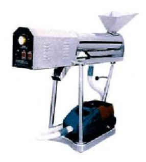
It is a new designed special purpose equipment for polishing the surface of capsules to improve the surface Smooth finish. Meets GMP standard.
