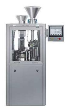
With an output of 400 capsules per minute, the processing range of the NJP-400C includes (micro) tablets, powders, pellets, and granules. It works with intermittent motion and doses powder via the proven tamping pin principle.
