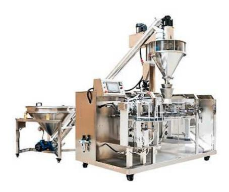
The premade bag automatic packaging machine replaces manual packaging, and realizes packaging automation for large enterprises and small and medium-sized enterprises. The operator only needs to put the finished bags one by one, and put hundreds of bags in the bag removal department of the equipment at a time. The mechanical claw of the equipment will automatically take the bag, print the date, open the bag, give a signal to the measuring device, and blank, seal, and output.
