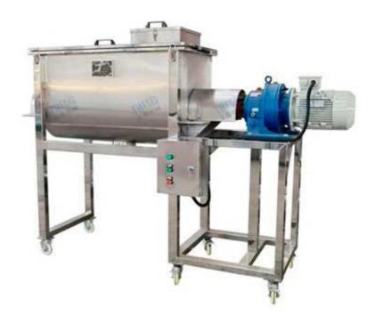
Adopted Full Stainless Steel 304 material, this dry powder mixing machine is designed with durable structure, long service life in various dry powder mixing processing.
