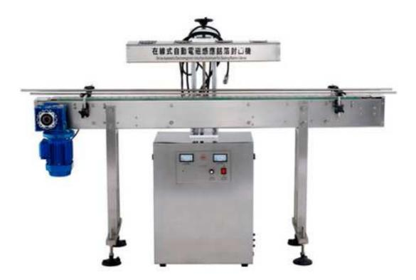
Conduction Sealing Machine uses the principle of electromagnetic induction to generate high temperature instantly on the aluminum foil on the bottle mouth, and then fuse the aluminum foil on the bottle mouth to achieve the function of sealing. It has good moisture-proof, mildew-proof, and anti-counterfeiting effects, thereby prolonging the storage time of items.
