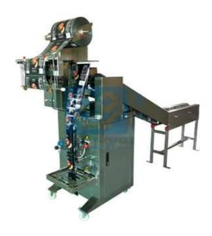
CE Series Automatic granular pillow bag packing machine This machine is suitable for packing non sticky, bulk or granular material, such as medical pills, food stuffs, plant seeds, washing powders, coffee, sugar desiccant, etc.
