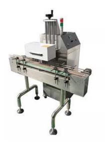
The bottles with aluminum foil pass under the inductive head in order, the aluminum foil get heated after receiving the energy produced by the inductive head. The heated aluminum foil melts the plastic film compounded and adheres tightly to the bottle mouth to obtain a sealing effect.
