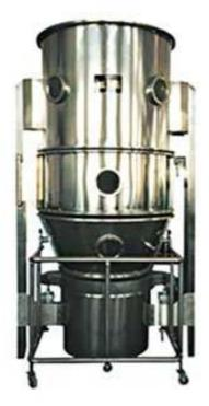
The machine is main used for drying powder or granules from pharmaceutical, foodstuff, chemical and so on industries.
