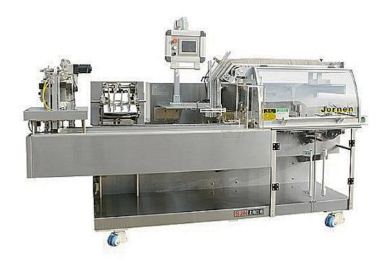
Automatic intermittent motion horizontal cartoning machine, very compact and reliable. The working area is in cantilever (balcony type) layout. The main structure has a vertical partition to separate the drive section (rear) from the operating zones (front). It is suitable for packaging of blisters, bottles, vials, pillow packs, etc.
