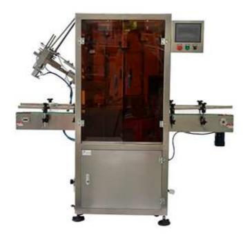
The CapperPacks Automatic Cap Sealing Machine is mainly suitable for sealing the dust-proof plastic caps of round bottles of various PET plastic, iron, aluminum and paper cans. It features advanced design, reasonable structure and simple operation.
