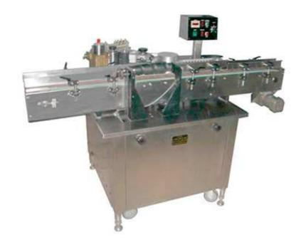
JHL-08 is suitable for small cylindrical container such as glass, plastic, PET bottle with precut paper label.
