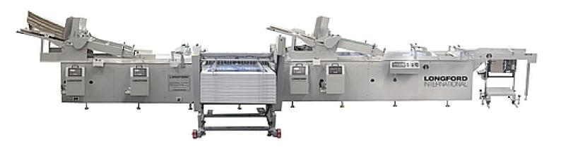
Design/build and install a complete turnkey large format poster collation and tipping system. A C750 feeds the large (up to 36"x40") backer card in the dual lugged conveyor, glue is applied across the backer card and the poster is tipped on using a VC200 vacuum feeder. The tipped on posters have glue applied to the outside edges and the matte frame is tipped on using another C750 feeder. The finished prints are then labelled and ready for sale.
