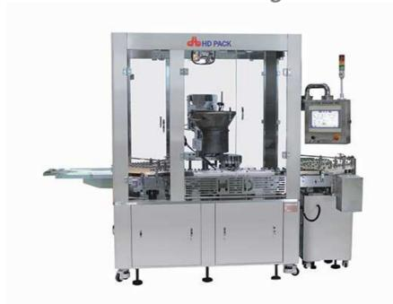
HD ACS Series are an automatic continuous motion machine suitable to seal cylindrical glass or plastic containers with alu-caps with or without plastic cover (Flip off/Tear off) by using fixed contrast balde. The position of the alu-caps feeding bowl is downstream to the sealing group thus minimizing the risk of aluminum particles contamination. HD ACS ensures perfect sealing of containers.
