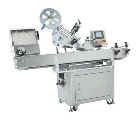
AL520 Horizontal Ampoule/Vial Labeler is suitable for many variety of tube labeling. When labeling, the tube will automatically rotate to allow the labeling device to apply the pressure for labeling. Suitable for medicine, food, beverage, and chemical industries. Can be used for plastic, glass, metal and other round containers/bottles. With its innovative design, its operation is so simple that even a primitive man can use.
