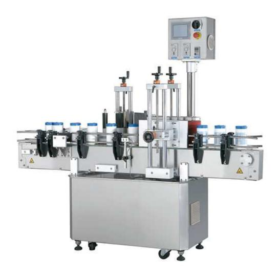
This Wrap Around Labeling Machine is designed for wrap-around labeling on cylindrical bottles and containers. It can be incorporated with a line or operated individually.
