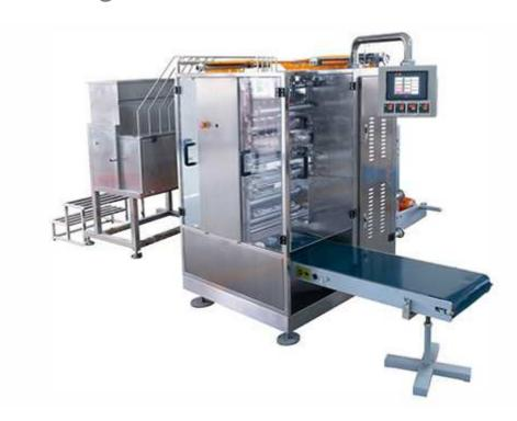
As shown in the picture, the packing machine is used for packing thick paste materials such as peanut oil, salad oil, tomato paste, cough syrup, shampoo, cream oil, vaseline and so on, providing measuring and automatic packing into sachets. It is used in the medicine, food, daily chemical industries, etc.
