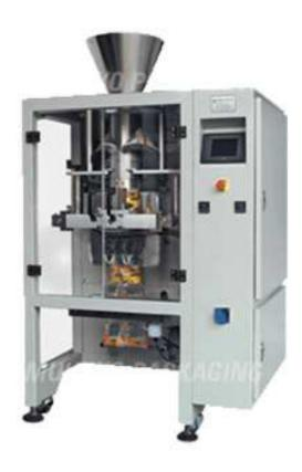
The MK-501 is a High speed servo diven vertical form, fill and seal (bagging) packaging machine designed to package granular and free flowing powdered products. This Servo driven Vffs packaging machine is equipped with high speed servo drive and it uses volumetric cup dosing system to produce center sealed pouches also commonly known as pillow pack or fin seal type pouches / bags.
