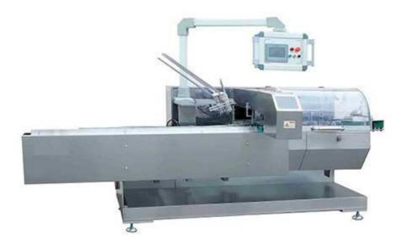
Automatic cooling patch packing machine is mainly used for packing of the cooling patch and collation 5 or 10 bags into the box. And it can also connect with the front printing equipment which will improve the capacity.
