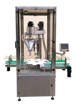
This series could do work of measuring, can holding, and can filling and etc, it can constitute the whole set can filling work line with other related machines, and suitable for filling kohl, glitter powder, pepper, cayenne pepper, milk powder, rice flour, albumen powder, soy milk powder, coffee powder, medicine powder, additive, essence and spice, etc.
