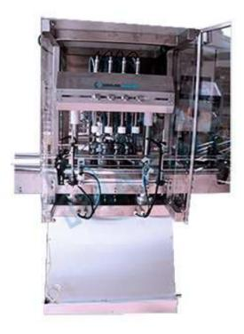
HMF 3000 Flowmeter filling Fast and high filling accuracy. Easy cleaning, suitable for high viscosity liquids and liquids. Filling volume differences between nozzles can be adjusted separately.
