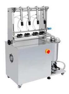
Designed for filling perfume into bottles and sealing the bottles afterwards. Minimum filling is 0.3 ml, maximal filling is 100 ml. Accuracy of filling is 0.05 ml. Production capacity is 1200-2000 bottles per hour. The machine can work with wide variety of bottle shapes and volumes.
