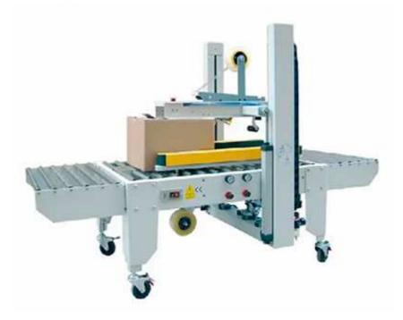
FX-5050Q is an automatic sealing machine that can automatically adapt to different carton sizes. The device can automatically sense and adjust the width and height, and is suitable for small batch and multi-specification production. This machine uses instant tape to seal the carton, which can complete the upper and lower sealing actions at one time.
